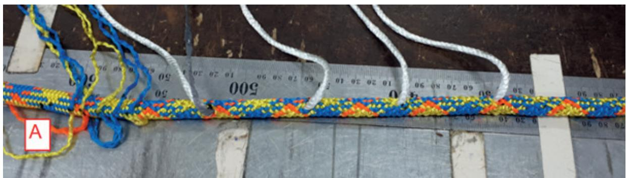
Milk the cover beginning at mark C. All cores should lie side by side within the cover. It's the best to milk the rope between your thumb and index finger, then you notice when the cores overlap/cross.
