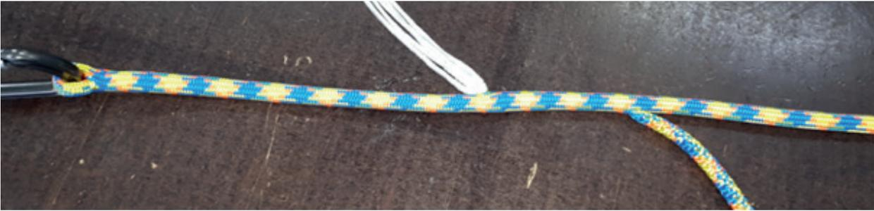
13. Mark the end of core and cover at mark C respectively D.
