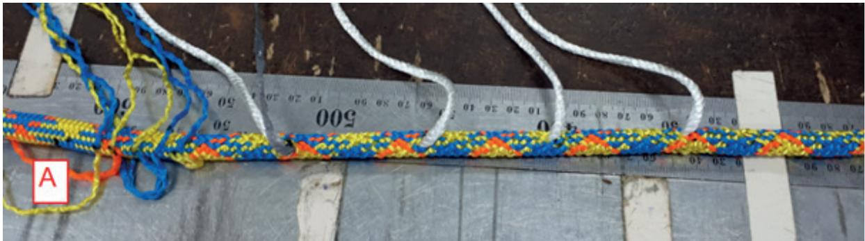
Milk the cover beginning at mark C. All cores should lie side by side within the cover. It's the best to milk the rope between your thumb and index finger, then you notice when the cores overlap/cross.
