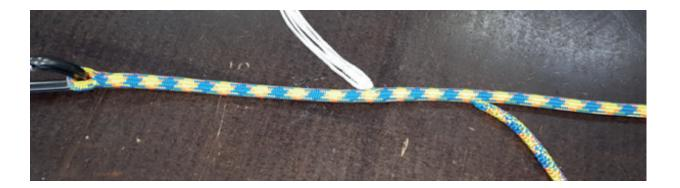
13. Mark the end of core and cover at mark C respectively D.
