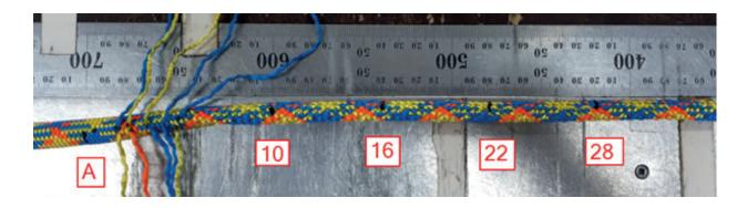
Pull out at every mark one of the cores, but don't cut them. Start with the core at the 10 cm mark.
