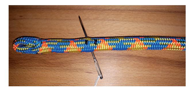
3. Pull the whipping twine through the rope until the end, melt it with a lighter and press it flat..
