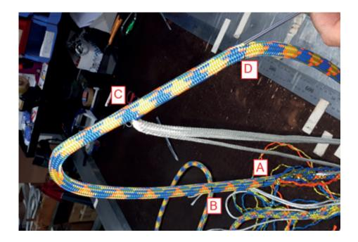
Important: don't push the wire sling through between the cores, always at the "ridge", to avoid that you have to pull the cover through some loops of the cores. It's easier when you push the wire sling through from bottom to top and the rope end is hanging down loose.
