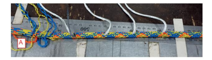
Milk the cover beginning at mark C. All core should lie side by side within the cover. It's the best to milk the rope between your thumb and index finger, then you notice when the cores overlap.
