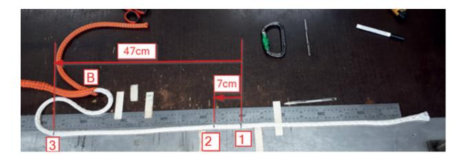
6. Beginning at mark 3 and mark each third crossing of the core yarns 3 times.
