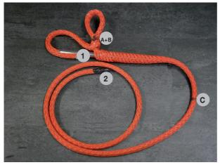
Pull tight and even out the rope at A/B.
