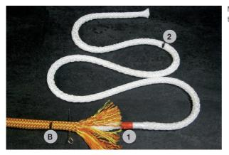
Mark 2 on the core at 37 cm from the rope end.
