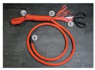
Pull out as much of rope end 1 as possible and fix with a needle near C. Remove 8 rope strands at equal distances and taper the rope end.
