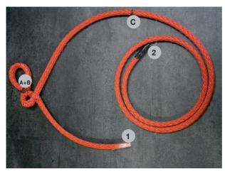
Pull rope end 2 through the rope just underneath the point where A and B meet.
