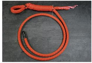
Remove the needle, even out the rope.
