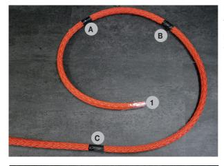
Mark A, B, C. 1 is the rope end near A. 2 is the other rope end. Measures according to table below. The distance between A and B defines the eye size.
