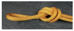
Tie a knot about 4 m from the rope end to prevent rope from moving.
