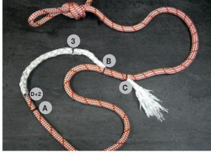
Even out cover and core. At mark C, where the core exits the cover, add a marking on the core. Pull the core out further, make a straight cut, unravel the rope end for 6 cm and taper the tip along those 6 cm.
