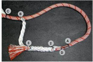
Pull the cover end (behind D) through the core from 2 to 3.
