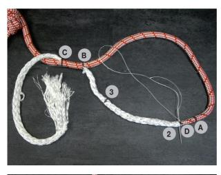
Bring section 2 to 3 back into position. D and 2 must be in the same place. Fix with two to three stitches using e.g. whipping twine of 0,5mm.
