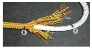
Taper the cover: Cut off half the yarns at 1,5 cm before B, cut another quarter of the yarns halfway and taper the remaining yarns until the end.
