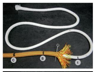
Pull out core and fix with a needle about 1,85 m from the rope end.
