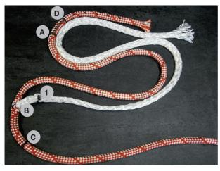
Pull out the core at B and mark the point of exit 1.
