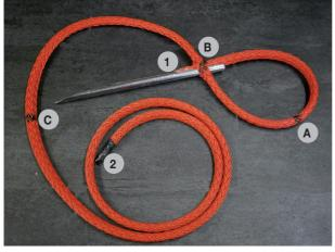
Pull the rope end 1 through the rope at B until A meets B.
