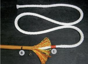
Cut intermediate cover at 1, remove the intermediate cover (from 1 to the rope end) and fix the cut end with adhesive tape.
