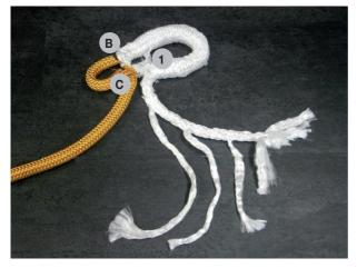
Pull core end out at mark 1 and taper along 30 cm: Remove 4 braids at equal distances, cut them off and taper the remaining rope end.
