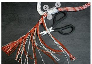
Pull the section 2 to 3 towards D as tightly as possible. Pull out the yarns marked before and cut them off for even tapering. Taper the remaining yarns at the tip.
