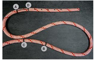
From D towards the rope end mark every fifth pair of yarns. Later on these marks are needed for cutting off the yarns for even tapering.
