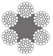
Stranded ropes are formed by laying the strands together helically, in one or more layers around a core. A high number of strands ensures a high flexibility and resistance to transversal pressure and wear. The compacted strands provide a smoother and bigger surface and create extended contact areas among the wires.
