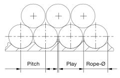
Figure 62 - Play = Pitch - Rope-Ø = (for a new applied rope)
