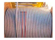
Figure 59 - relationship between pre-tensioning and D/d ratio of the drum
