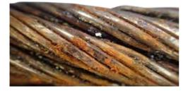
Figure 79 - External corrosion
