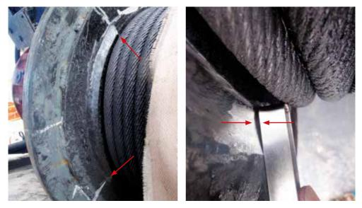
Figure 54 - Constriction that can cause rope distractions
