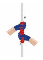
Figure 71 - manual lubrication located at sheave (symbolic illustration) Figure 72 - manual lubrication with greased cloth (symbolic illustration)
