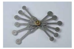
Figure 33 - Sheave gauges
