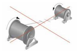
Figure 44 - incorrect tensioned unwinding using a winch
