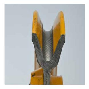
Figure 36 - negative impression of a used sheave
