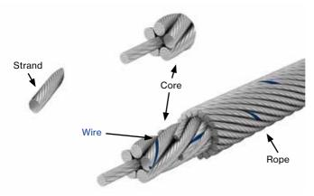
Figure 1 - Elements of a wire rope
