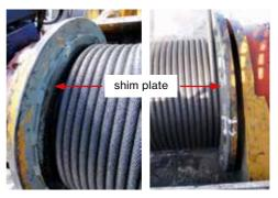
Figure 52 - shim-plate on drum
