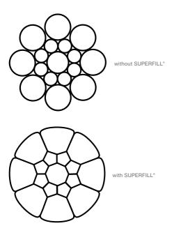
Figure 4 - SUPERFILL® compaction technology
