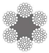
Figure 5 - Fiber cores (FC)
