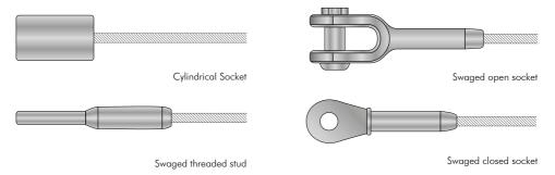
Figure 21d - Swaged steel fittings
