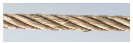
Figure 88 - Wire protrusion in loops
