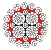
Figure 10 - High performance rope
