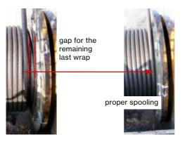
Figure 53 - proper spooling of first layer in order to avoid gaps to shim-plates that can cause rope crushing
