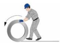
Figure 39 - proper unwinding off a coil
