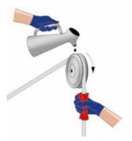
Figure 70 - automated lubrication located at sheave (symbolic illustration)
