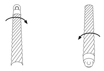
Figure 56 - example of a dead end: two different views, but one rope Figure 57 - Lay Type of rope: ordinary right
