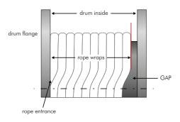
Figure 51 - gap check after first layer fully spooled on sheave
