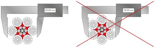
Figure 29 - Checking the diameter
