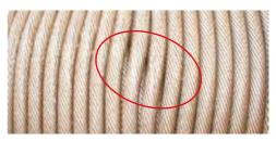
Figure 67 - loose spooling of rope in the outer layers
