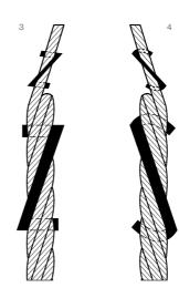
3 Right Hand Lang Lay (zZ or RHLL) 4 Left Hand Lang Lay (sS or LHLL)
