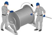
Figure 41 - correct unwinding off a bobbin
