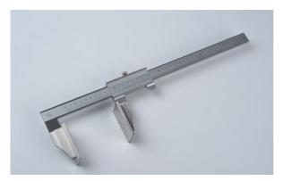
Figure 30 - Sliding calipers with wide plates
