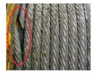
Figure 50 - entrance of the rope on the drum
