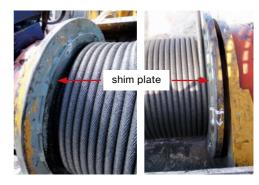
Figure 52 - shim-plate on drum
