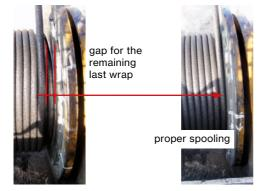
Figure 53 - proper spooling of first layer in order to avoid gaps to shim-plates that can cause rope crushing
