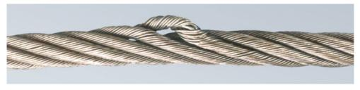
Figure 87 - Strand protrusion/distortion
