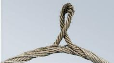
Figure 85 - Core protrusion
