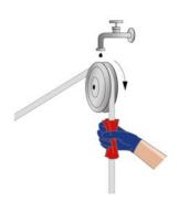
Figure 70 - automated lubrication located at sheave (symbolic illustration)
