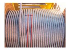
Figure 60 - Proper spooling (no gap between the wraps)
