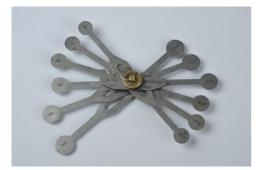
Figure 33 - Sheave gauges
