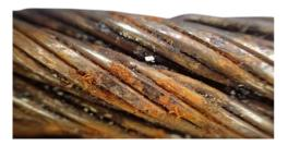
Figure 79 - External corrosion
