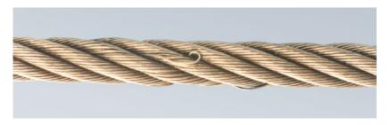
Figure 88 - Wire protrusion in loops
