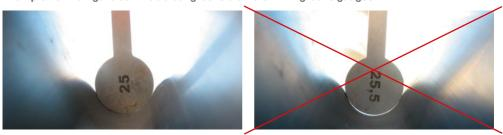
Figure 34 - act. groove diameter 25.0mm
