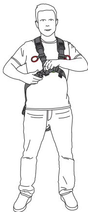
Feed the lock of the smartlock buckle through the front ring. Close the smartlock buckle (see 2.a.)
