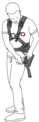
Close smartlock buckles in the leg loops (See 2.a.)
