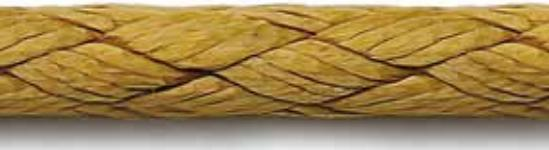
To obtain the outstanding performance level of PBO, it is recommended to use a protective cover. Properties like highest breaking load, very low elongation and zero creep need to be preserved by a solid cover to hinder degrading caused by UV and other environmental influences.
