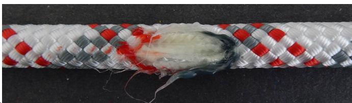
Pic.5: Patron Plus 11mm at 250°C for 1 min
