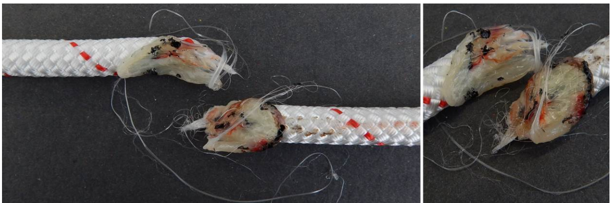
Pic.6: Patron 11mm – Rope break at 300°C
