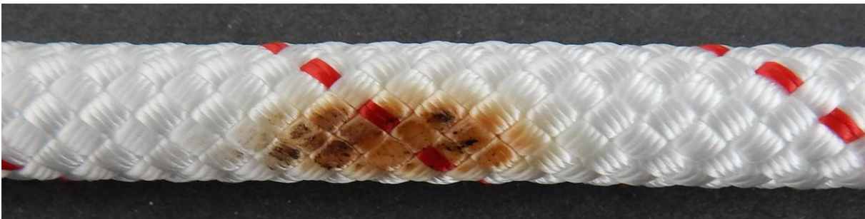
Pic.3: Patron 11mm at 210°C for 20 min
