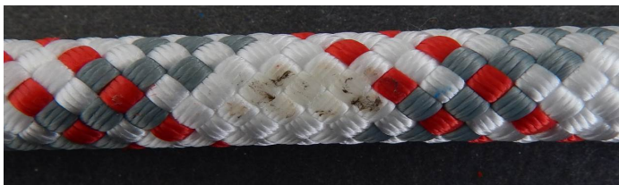
Pic.4: Patron Plus 11mm at 230°C for 1 min.
