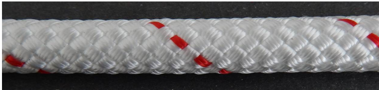
Pic.1: Patron 11mm – after gasoline influence for 15 min
