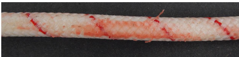
Pic.2: Patron 11mm – after battery acid influence for 5 min.
