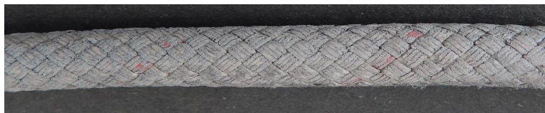
Pic.3: Patron 11mm – covered with corrosion protection paint
