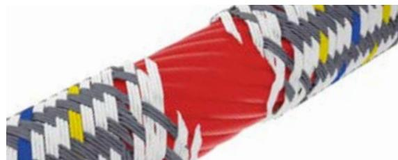
In effect since 2017, the FEM 5.024 standard defines guidelines, particularly regarding the point of discard for the safe use of high performance fiber ropes on cranes. At the time when the point of discard has been reached, soLITE®, thanks to its construction, still has 100 % of its breaking load. This makes soLITE® even safer than a steel wire rope.
