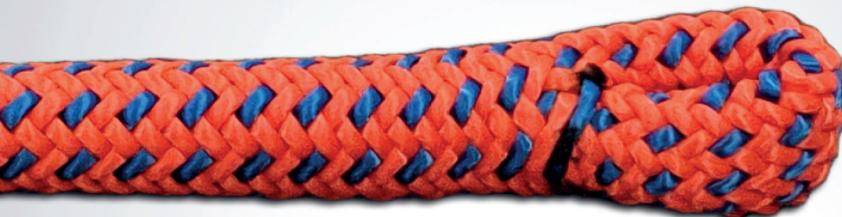
11. Push the cover end with a splice needle from mark 2 to mark 3.
