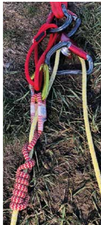
Fig 2. Valdotain Tresse VT Prusik on TEC REEP low angle system, being changed over with optional karabiner below pulley across both ropes to assist with Prusik minding during haul. In this photo the 80cm Tendon Timber Prusik was used, however the author recommends using the 100 or 120cm variant instead to remove the additional off-set prusik sling as illustrated.
