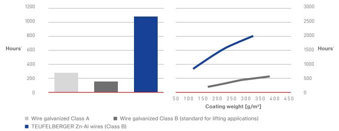
\*Hours of salt spray test until the appearance of 5% dark brown rust (DBR).
