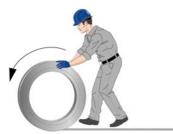
Figure 39 - proper unwinding off a coil
