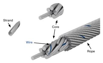
Figure 1 - Elements of a wire rope
