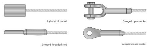
Figure 21d - Swaged steel fittings
