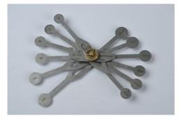
Figure 33 - Sheave gauges
