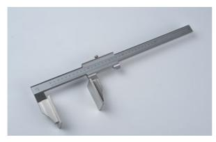
Figure 30 - Sliding calipers with wide plates
