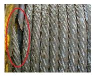
Figure 50 - entrance of the rope on the drum
