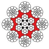
The steel wire rope core can be covered with solid polymer (EPIWRC) – Teufelberger-Redaelli PLASTFILL<sup>®</sup> technology.
