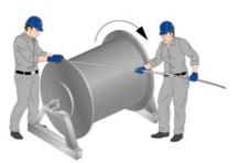
Figure 40 - improper unwinding off a coil
