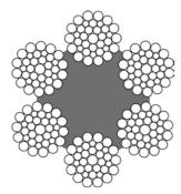
Figure 5 - Fiber cores (FC)
