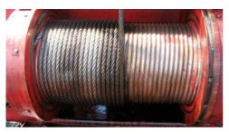
Figure 68 - drum ground should be visible for proper measurement
