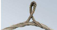
Figure 85 - Core protrusion
