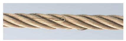
Figure 88 - Wire protrusion in loops
