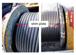
Figure 52 - shim-plate on drum
