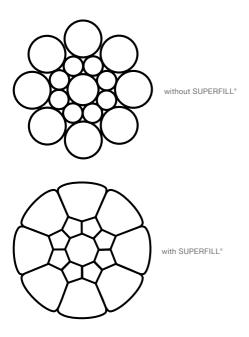
Figure 4 - SUPERFILL® compaction technology
