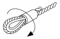
Figure 61 - how to untwist a hoisting rope
