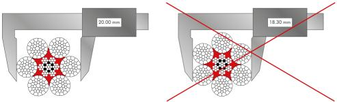
Figure 29 - Checking the diameter
