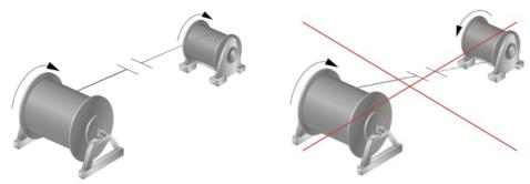
Figure 43 - correct tensioned unwinding using a winch
