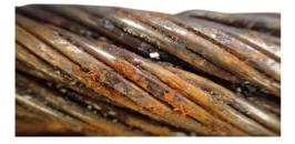
Figure 79 - External corrosion
