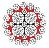
Figure 10 - High performance rope
