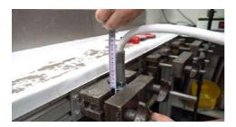
Measure the length of the grouting sleeve.
