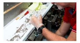
2) Pull the grouting brush into the grouting sleeve until adhesive tape appears at the bottom of the hole. In order to reduce leakage of the resin onto the rope, Teufelberger recommends sealing the transition between the grouting and the rope sheath in this position once again with an additional adhesive tape.
