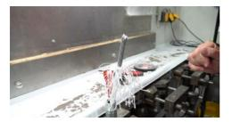
**Cut** the rope straight with a knife/scissors and push the grouting cone over the rope until it protrudes approx. 5 mm beyond the grouting cone.
