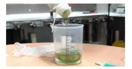
**Mix** the pre-dosed components resin + hardener together in the mixing bowl. Stir for approx. 2 minutes.
