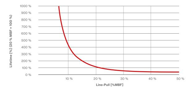
An MRT operating 100.000 cycles with a line-pull of 10 tons runs 1.000.000 ton-cycles. Another MRT operates 20.000 cycles with a line-pull of 50 tons runs also 1.000.000 ton-cycles. Theoretically, the ton-cycles are equal in both cases, but in reality the cycles with a higher line-pull causes more damage to the rope than those cycles with the lower line-pull. Hence this example shows the limited applicability of the ton-cycle approach.
